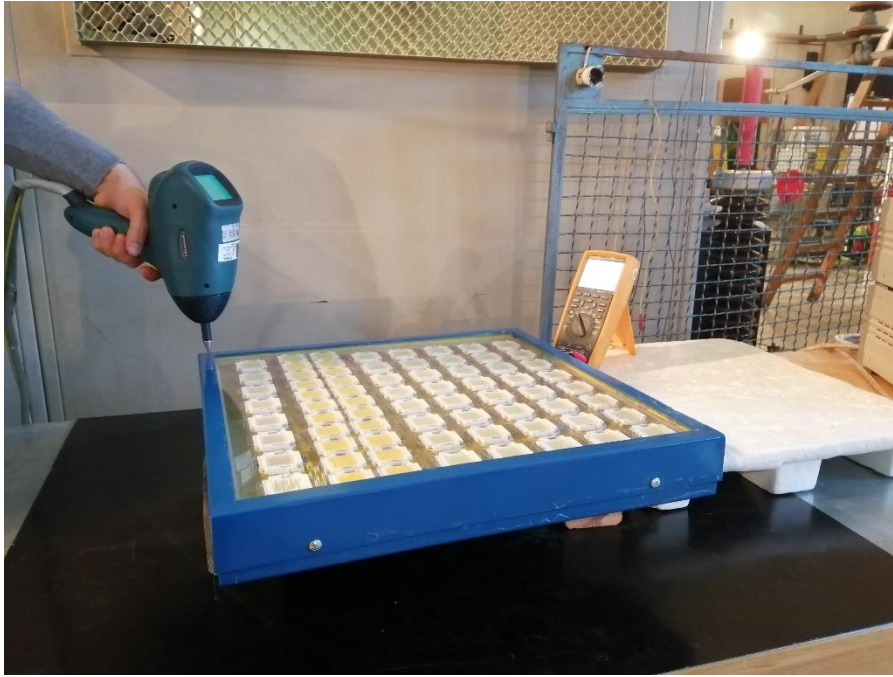
Photo 9.1: Setup for electrostatic discharge test
