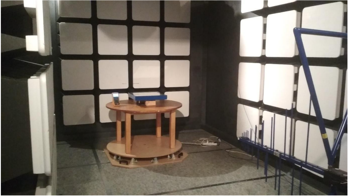
Photo 8.1: Setup for radiated emissions test (30MHz-1GHz)
