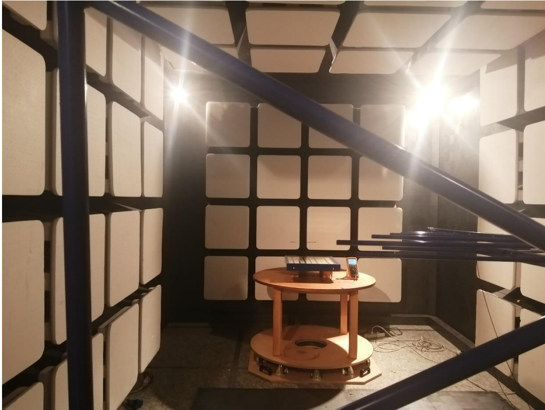
Photo 10.1: Setup for RF electromagnetic field test (80MHz-1GHz)
